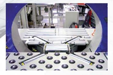
The twist wrapping machine was developed to apply a semi-automatic solution for wrapping ringshaped products such as tires with packaging material (typically stretch film) in a spiral mode.
