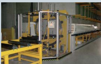
Inline solution for complete packs of laminated beams. Additional bandages to save the manual strapping
