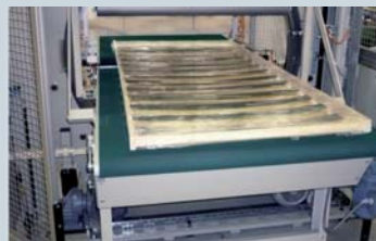
Packaging of slatted frames with semi and fully automatic machines
