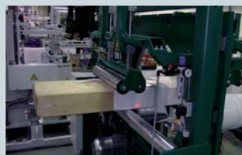
Wrapping of single bars with highspeed application up to 60 m/min
