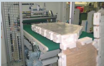
Automatic wrapping of table tops or working tops with corner protection
